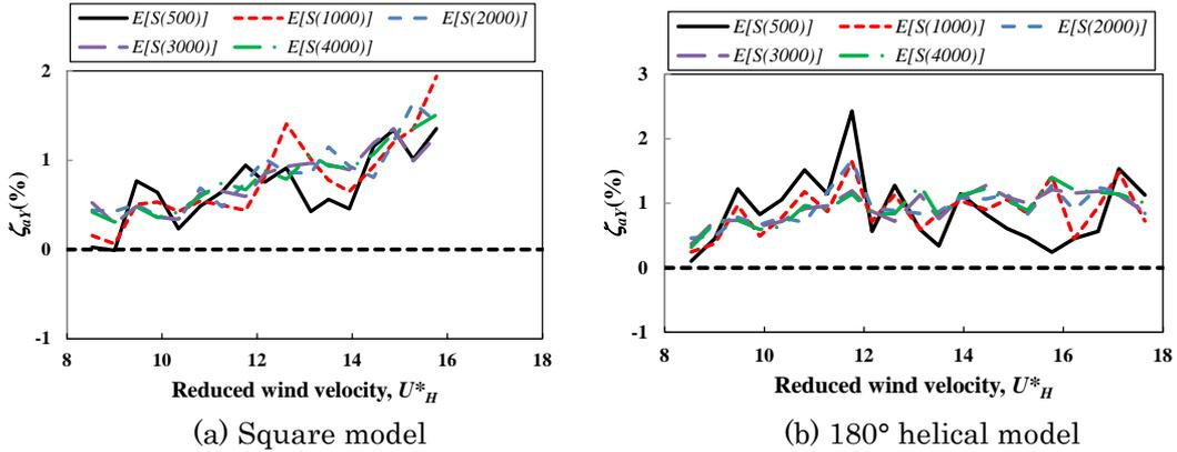
Fig. 4 Effect of the time segments in estimating the aerodynamic damping ratio in the along-wind direction
