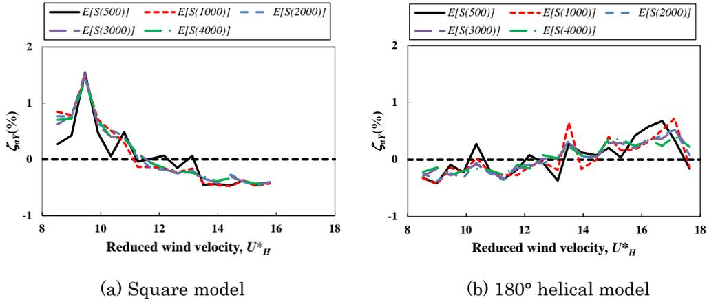
Fig. 5 Effect of the time segments in estimating the aerodynamic damping ratio in the across-wind direction
