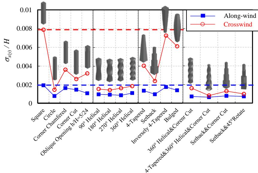
Fig. 3 Normalized rms displacements on super tall building at design wind speed
