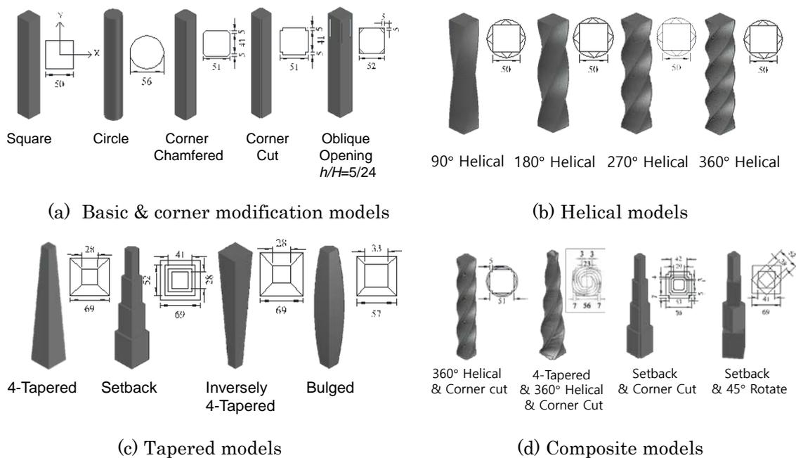
Fig. 1 Rocking vibration models
