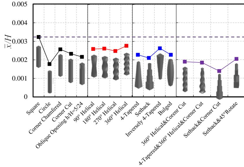
Fig. 2 Normalized mean displacements on super tall building at design wind speed
